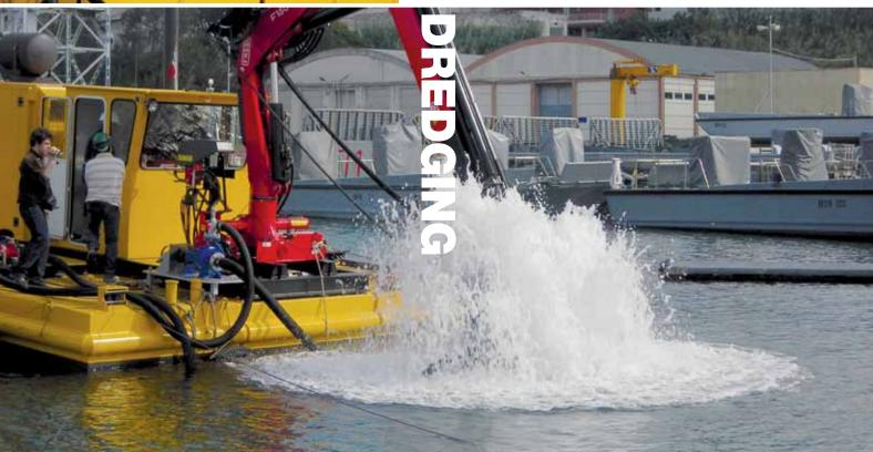
Dragflow hydraulic pumps are ideal to fill-up geotextiles. Thanks to variable rotation speed of the pump the system production can be easily adjusted in order to guarantee best mixing with eventual polymer and optimize fill-up cycles.
